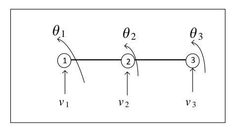
The stiffness matrix for each element is found and then the global stiffness matrix is assembled. Then  $\{p_{global}\}=[K_{global}]\{d_{global}\}$  is solved as before. The first step is to move all loads to the nodes as was done before. This is done for each element. The formulas for equivalent loads remain the same, but now L becomes L/2. The following diagram show the equivalent loading for P
