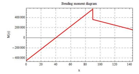
The reason for this is because the solution v(x) obtained using the finite elements method is a third degree polynomial and after differentiating twice to obtain the bending moment  $(M(x) = -EI\frac{d^2v}{dx^2})$  the result becomes a linear function in x while in the analytical solution case, when the load is distributed, the solution v(x) is a fourth degree polynomial. Hence the bending moment will be quadratic function in x in the analytical case.
