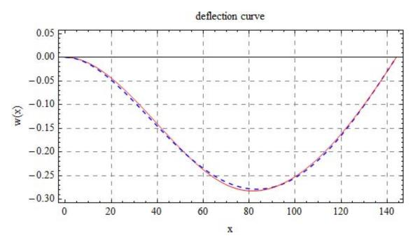
In the above, the blue dashed curve is the analytical solution, and the red curve is the finite elements solution using 2 elements. It can be seen that the finite element solution for the deflection is now in a very good agreement with the analytical solution.
