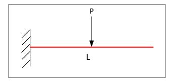
In using stiffness method, all loads must be on the nodes. The vector  $\{p\}$  is the nodal forces vector. Hence equivalent nodal loads are found for the load in the middle of the beam. The equivalent loading is the following
