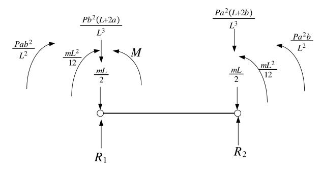
Now that all loads are on the nodes, the stiffness equation is applied
