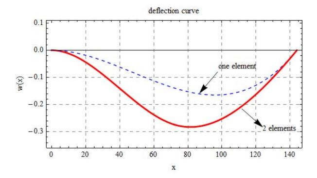
The analytical deflection for the beam in problem three above (fixed on the left and simply supported at the right end) when there is uniformly loaded with w lbs per unit length is given by
