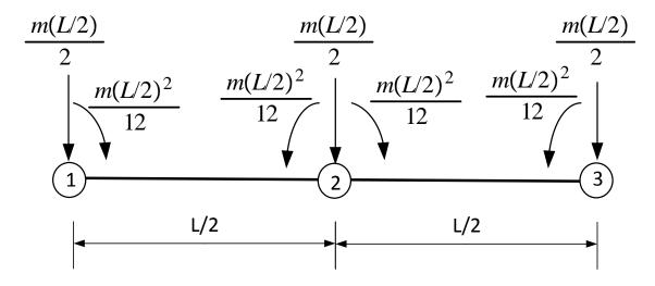
Now the above two diagrams are put together to show all equivalent loads with the original reaction forces to obtain the following diagram
