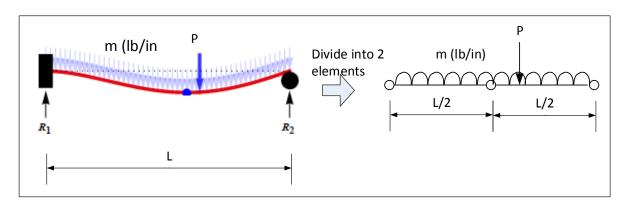
There is 6 total degrees of freedom. two at each node. Hence the stiffness matrix for the whole beam (including both elements) will be 6 by 6. For each element however, the same stiffness matrix will be used as above and that will remain as before 4 by 4.
