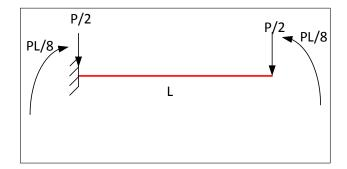
Now that equivalent loading is in place, we continue as before. Making a free body diagram showing all loads (including reaction forces)
