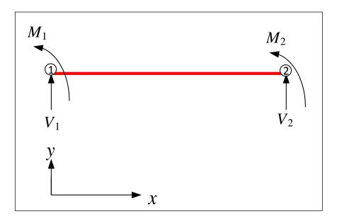
The above diagram shows the signs used for the applied forces direction when acting in the positive sense. Since this is a one dimensional problem, the displacement field (the unknown being solved for) will be a function of one independent variable which is the x coordinate. The displacement field in the vertical direction is called v(x). This is the vertical displacement of point x on the beam from the original x - axis. The following diagram shows the notation used for the coordinates.
