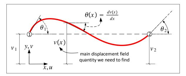
In the direct method of finding the stiffness matrix, the forces at the ends of the beam are found directly by the use of beam theory. In beam theory the signs are different from what is given in the first diagram above. Therefore, the moment and shear forces obtained using beam theory ( $M_B$  and  $V_B$  in the diagram below) will have different signs when compared to the external forces. The signs are then adjusted to reflect the convention as shown in the diagram above using M and V.
