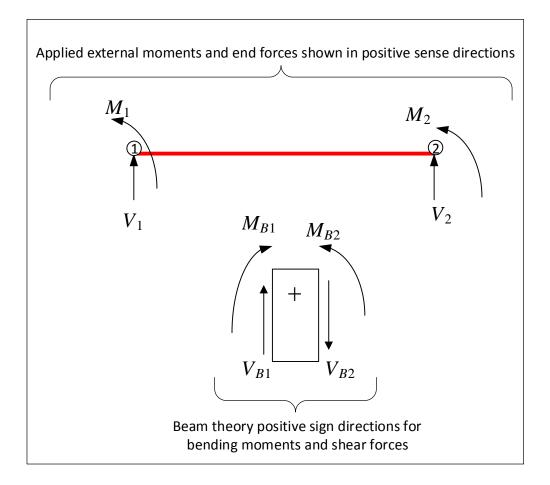
The goal now is to obtain expressions for external loads  $M_i$  and  $R_i$  in the above diagram as function of the displacements at the nodes  $\{d\} = \{v_1, \theta_1, v_2, \theta_2\}^T$ .
