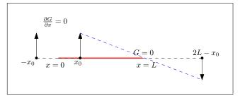
But now we see that the image at  $x = -x_0$  has affected condition of G = 0 at x = L and will make it not zero as we wanted. So to counter effect this, we have to add another negative image at distance  $x = 2L + x_0$  to cancel the effect of the image at  $x = -x_0$ . We end up with this setup
