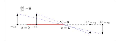
But now we see that the two negative images we added to the right will no longer make  $G_x(0, t) = 0$ , so we need to counter effect this by adding two negative images to the left side to keep  $G_x(0, t) = 0$ . So we end up with
