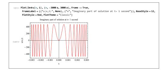
We see the rapid oscillations as distance goes away from the origin. This is due to the  $x^2$  term making the radial frequency value increase quickly with x. We now plot the  $|u(x,t)|^2$ . Looking at solution in (9), and since complex exponential is  $\pm 1$ , then the amplitude is governed by  $\sqrt{\frac{2}{\pi\lambda t}} \cos\left(\frac{2\pi a}{\lambda}\frac{x}{t}\right)$  part of the solution. Hence
