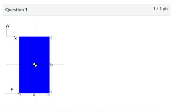
A rectangular body with mass 3 kg, width a=0.3 m and height b=0.7 m as seen above is acted upon by a force F=30 N in the bottom corner in the x-direction as seen above. The body lies on a horizontal plane. The center of gravity is at the geometric center of the object.
