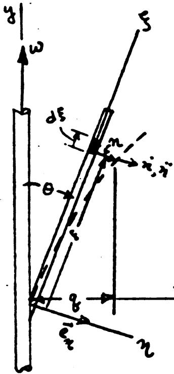
"Steady State" shape of a rotating rod
