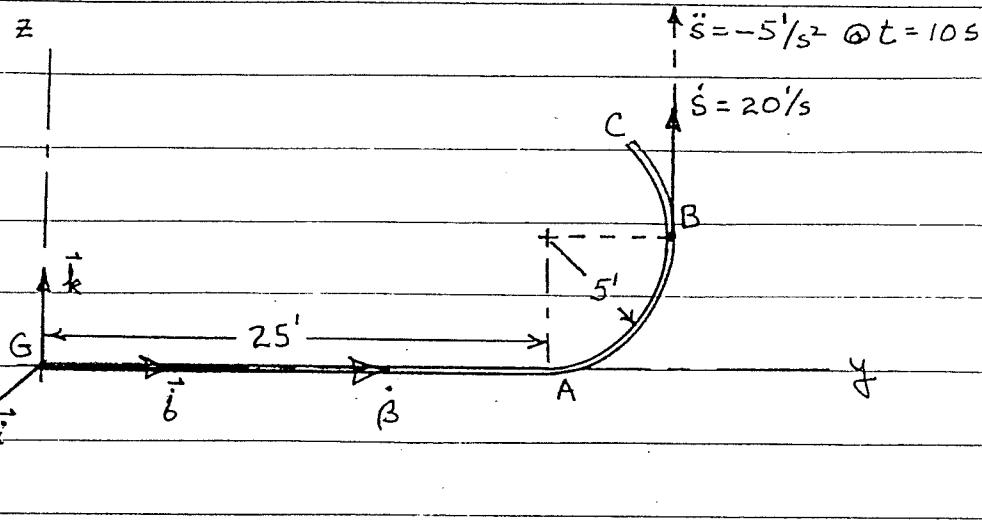
$$\vec{v}_G = 200 \vec{j} + 3t \vec{k} \text{ (ft/s)} = (v_{G,y}) \vec{j} + (v_{G,z}) \vec{k}$$
