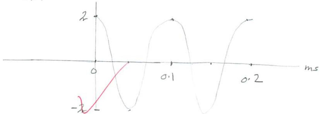
ⓑ  $F(m(t)) = \frac{A_m}{2} [\delta(f-f_m) + \delta(f+f_m)] \quad \text{where } A_m = 2 \text{ here.}$
