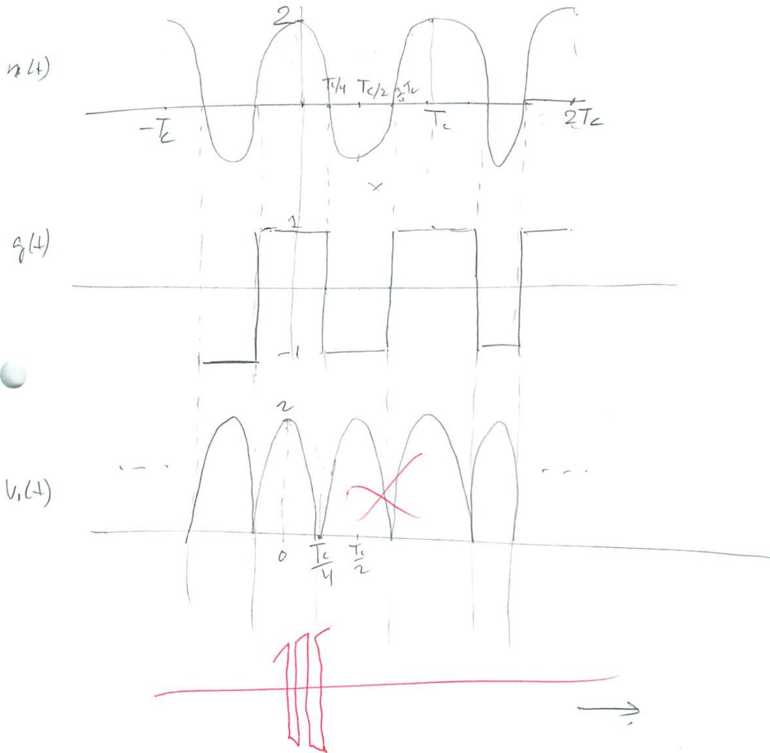
(5) the spectrum of  $v_1(t)$  is  $F(m(t)) \otimes F(g(t))$  (4)
