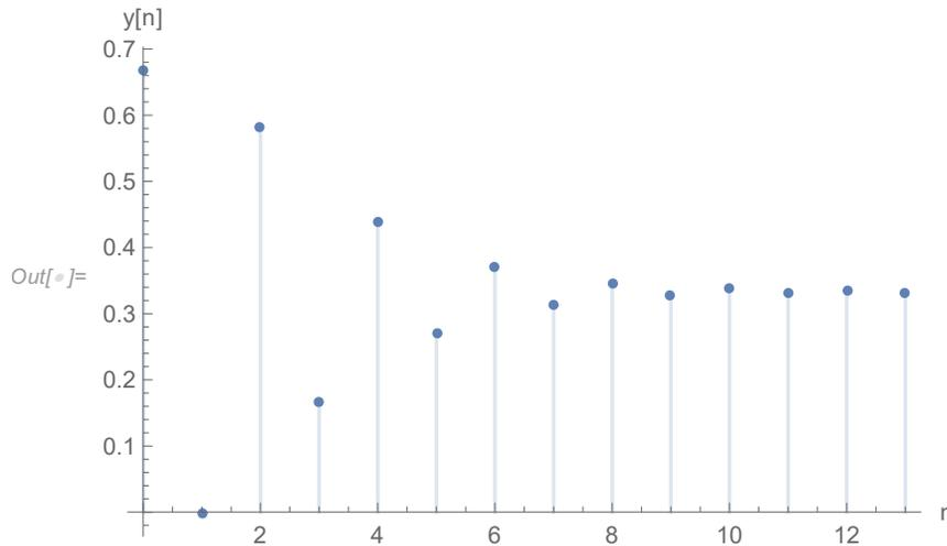
Figure 4: Plot of reponse  $y[n]$  to step input
