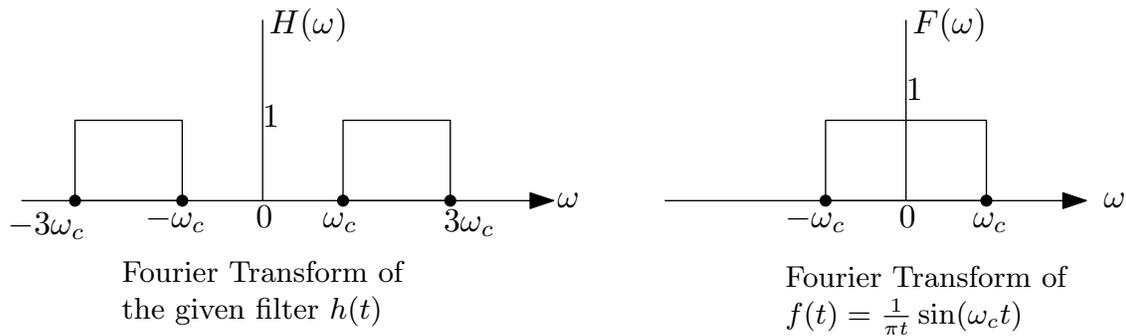
Figure 1: Sketch of CTFT of filter and sinc function
