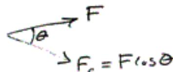
$$\text{so } dF_c = \frac{\partial F_c}{\partial F} dF + \frac{\partial F_c}{\partial \theta} d\theta$$
