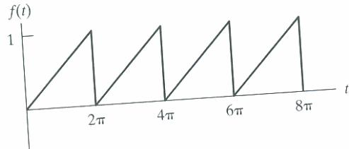
Figure P3.29 Sawtooth periodic signal.
