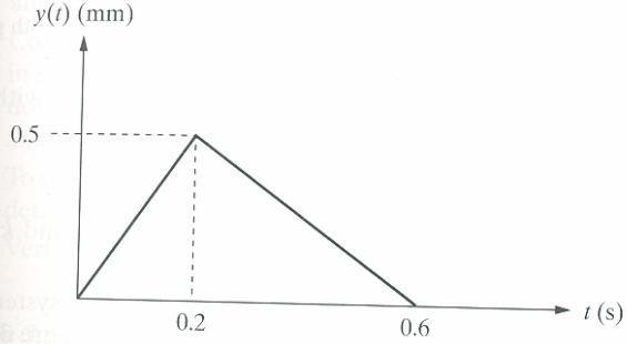
**Figure P3.21** Triangular pulse input.
