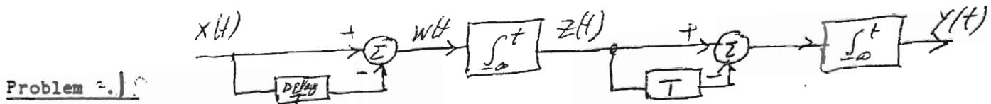
The first integrator input is equal to  $x(t) - x(t-T)$ . The Fourier transform of this input signal is  $[1 - \exp(-j2\pi fT)]X(f)$ . The value of this transform is zero at  $f=0$ . It follows therefore that the Fourier transform of the first integrator output is equal to
