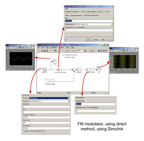
The MDL file is fm\_modulate\_direct.mdl
