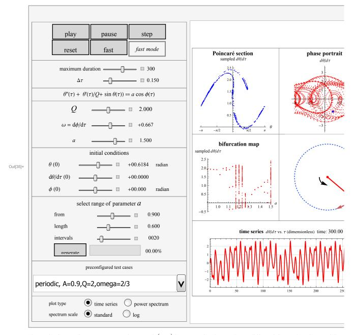
Theory background:  $\theta'' + c \theta' + g/L \sin \theta = A \sin(\omega_f t)$  is a second-order nonlinear differential equation that models the motion of a simple pendulum subject to a forcing function  $A \sin(\omega t)$ , where c is the damping coefficient, L is the length of the pendulum, and  $\theta$  is its angular position.
