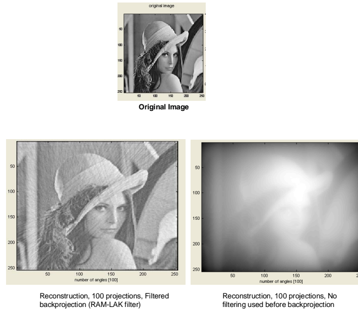
Figure 20: Effect of ram lak filter
