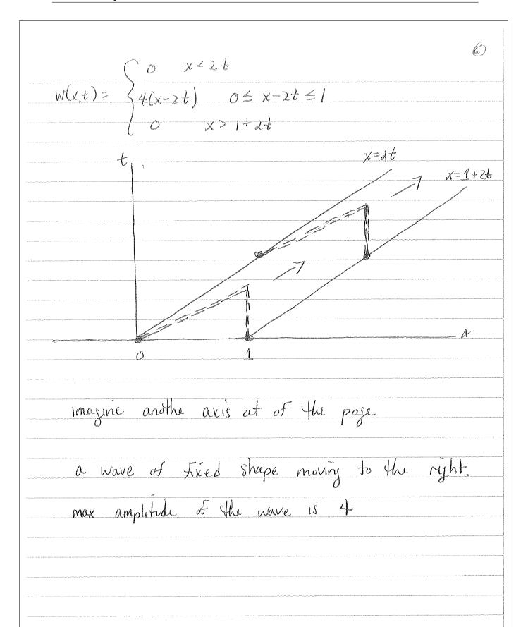
Simple Application: Transport with Decay Transport of a radioactively decaying solve in a uniform flow with wave spaced c  $\frac{\partial u(x,t)}{\partial t} + c \frac{\partial u(x,t)}{\partial x} = -a u(x,t) \qquad u(x,0) = f(x)$ - & < x < & [f(x) given for all values of the argument a > 0 is the decay rate ulx,t) is concentration [amount per init valurne]
