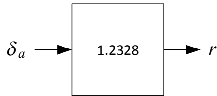
Figure 2.39: G_{v, \delta_a} block diagram for problem 2
