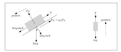
The acceleration of each body is the same. Let this acceleration be a. From the above free body diagram of the 2m body the equation of motion is now derived (using positive direction as show)
