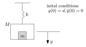
The block of mass m will leave the floor of the box when the vertical acceleration is large enough to match the gravity acceleration g. The equation of motion of the overall system is given by
