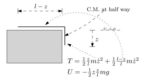
The top portion of the rope moves with same speed as the hanging portion. Hence z is used to describe the motion as the generalized coordinate. From the above
