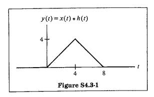
(b) The convolution can be evaluated by using the convolution formula. The limits can be verified by graphically visualizing the convolution.
