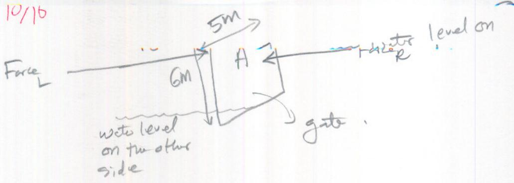
a gate of area  $A$  ( $5 \times 6 \text{ m}^2$ ). on one side, water has pressure on wall. on the other side, we have air pressure. need to find net horizontal force on gate.
