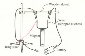
A. On an enlargement of the figure below, sketch field lines representing the magnetic field of the bar magnet. Show the field both inside and outside the magnet.
