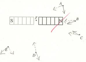
Compare the field vectors for the two half-stacks of magnets to the field vectors for the whole stack.
