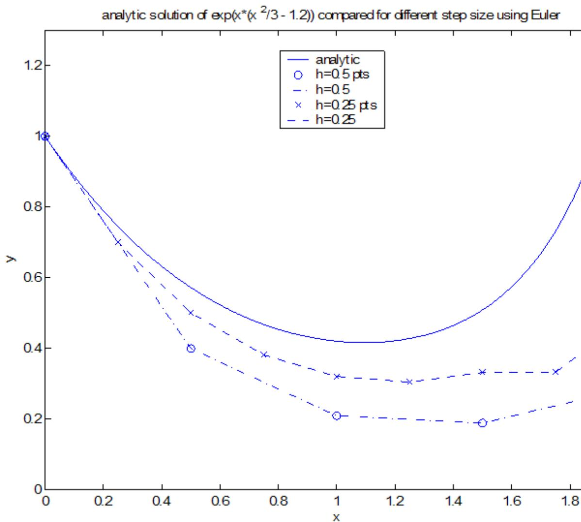
Notice that as step size  $h$  is decreased, the numerical solution is becoming closer to the analytical solution.
