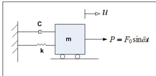
Hence the equation of motion can now be written from the free body diagram as (where  $M$  is the mass of the electric motor) and assuming the mass is moving to the right, and taking  $u$  relative to the static equilibrium position.
