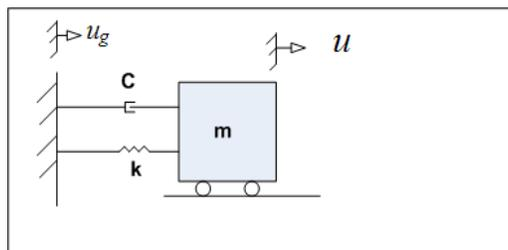
Where in the above,  $u$  is the absolute displacement of the tower, and  $u_g$  is the absolute displacement of the ground. The free body diagram is
