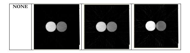
NOISE ADDED. Showing cross talk at time frame 4 as the window size was changed. Noise is Gaussian with zero mean and 5% S.D. of maximum projection signal.
