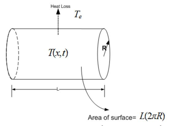
Hence lateral heat loss rate between x = a and x = b is  $\left[ -\int_a^b k \, dx \, (2\pi r) \, (T(x,t) - T_e) \right]$ . The minus sign is to say that this is considered to be a heat loss, not gain, into the volume under consideration. Now need to find what the units of this k is (this is NOT the heat conductivity coefficient). Using dimensional analysis, we write
