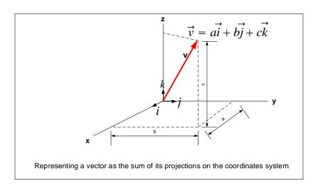
Now that we know how a vector is represented by adding its projections along the direction of each base vector, we are ready to make the switch to a new and exciting world, where vectors become functions and the number of basis instead of being fixed at 3 become very large, in fact, it become infinitely large. This new vector space is called the Hilbert space.
