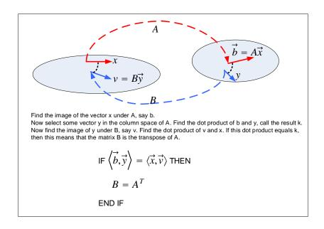
Now let us try to apply the above diagram to find the adjoint operator we need. Instead of using the Matrix notation of A and  $A^T$ , we now use the notation of L and  $L^*$ , where here  $L^*$  is the adjoint operator of L. Hence we seek to find an operator  $L^*$  such that  $\langle Lf,q\rangle=\langle f,L^*q\rangle$
