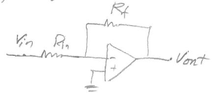
$$V_{out} = -V_{in} \left( \frac{R_f}{R_{in}} \right)$$
