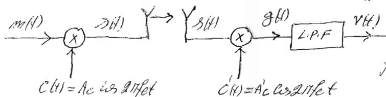
fig # (2) Coherent detection of DSB-SC.
