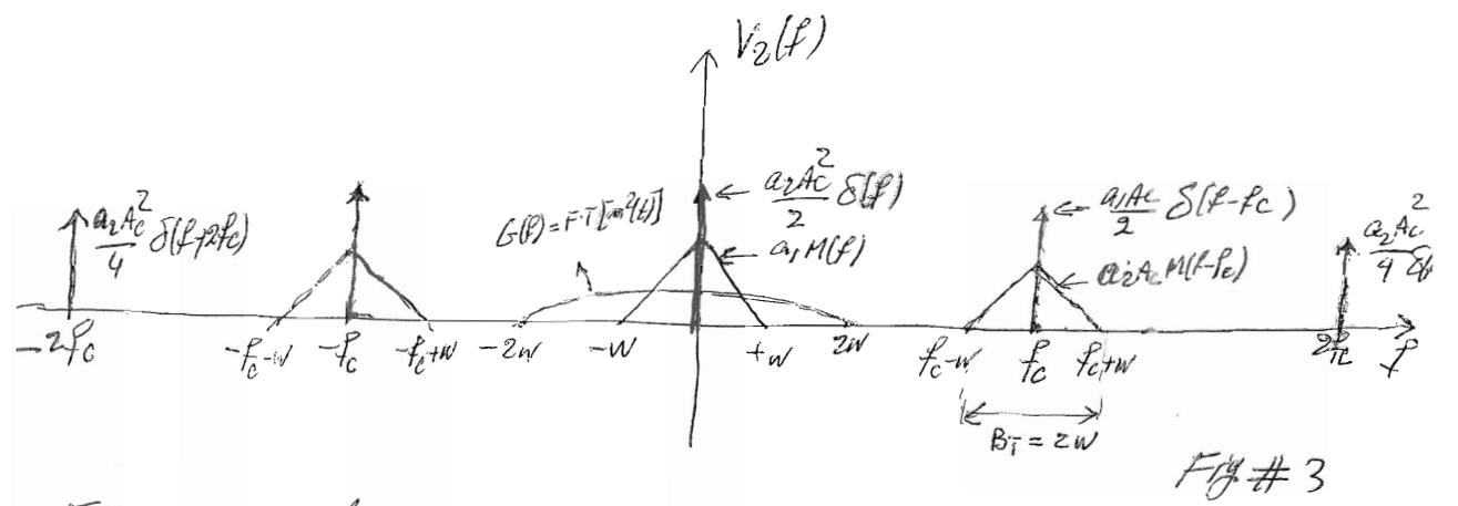
FIG # 3 Shows the spectral content of  $V_2(t)$ .
