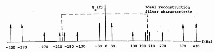
From this diagram, we deduce that in order to recover the original signal g(t) from its sampled version, the low-pass reconstruction filter must have a cutoff frequency greater than 190 Hz but less than 210 Hz.
